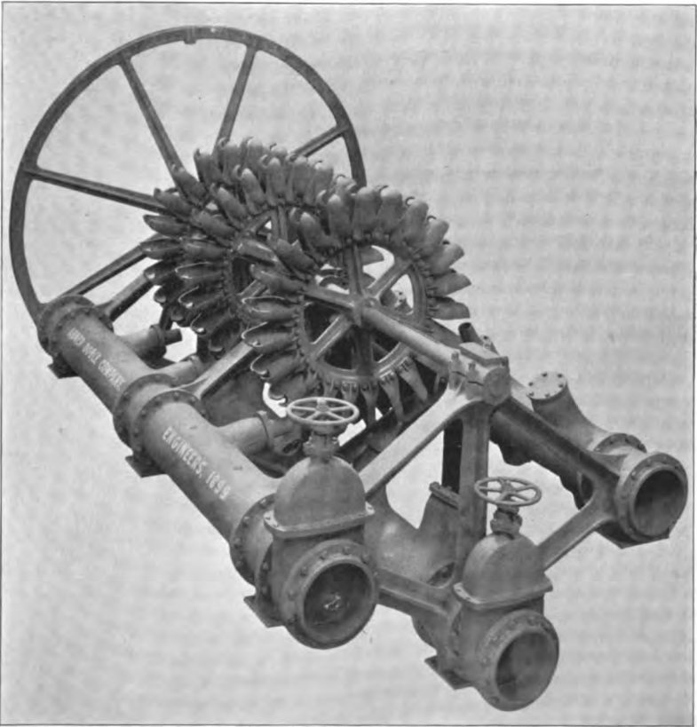
150 HORSE-POWER TANGENTIAL WHEEL. 35 FOOT HEAD, 90 REVOLUTIONS PER MINUTE.
