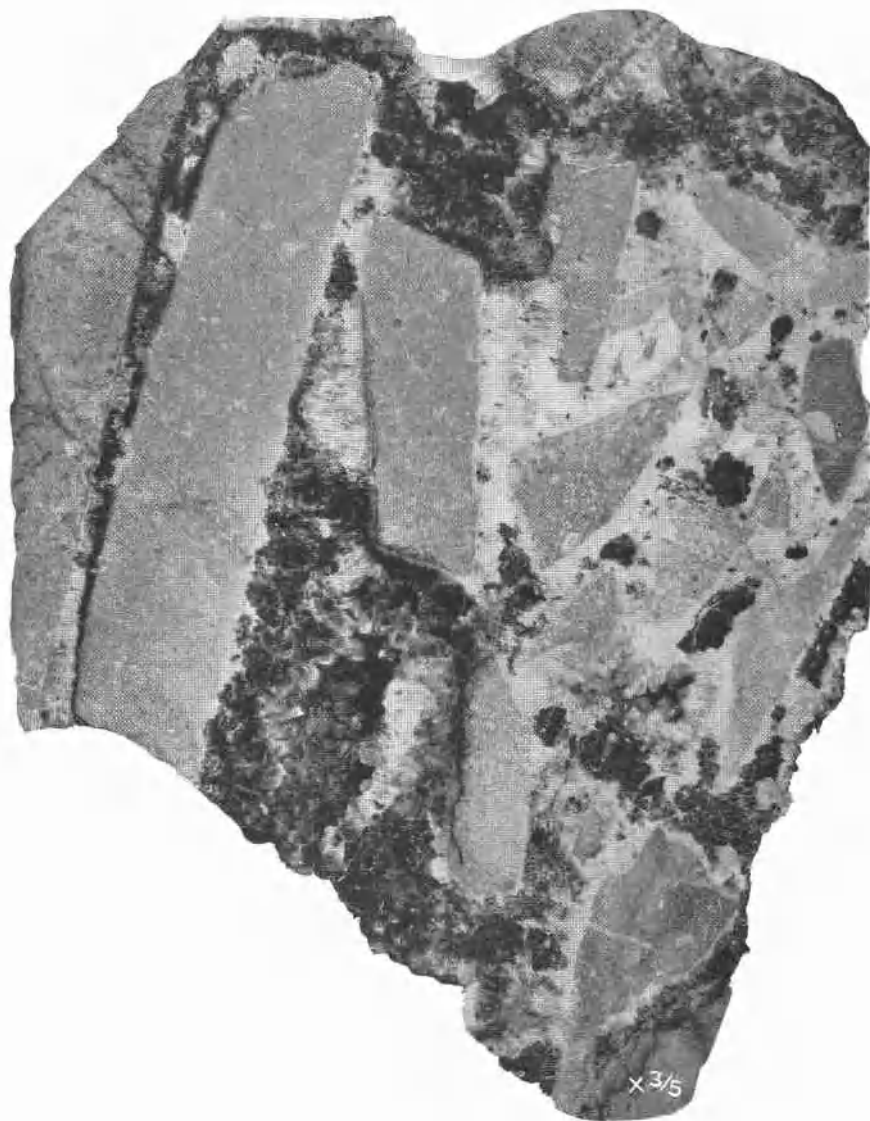
TYPICAL VEIN BRECCIA OF PARTLY ALTERED LABRADORITE ANDESITE IN SHARPLY ANGULAR FRAGMENTS CEMENTED BY VUGGY COMB QUARTZ CONTAINING SCATTERED SULPHIDES.
