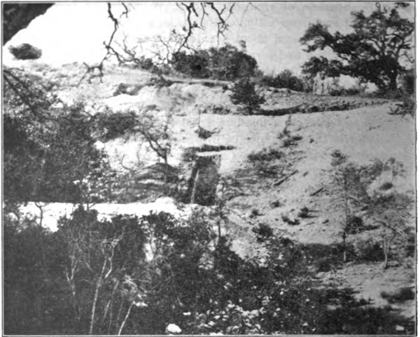
Dolomite Deposit, 11 miles from Hollister, San Benito County, showing method of tunneling into the deposit to avoid overburden and the impure upper portion of deposit.
