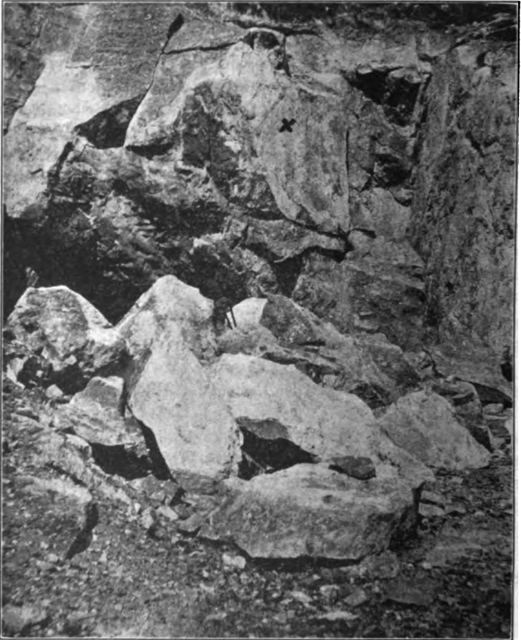
Photo No. 48. Three Colored Marble Quarry—showing large broken blocks at face of quarry. The block marked X measures roughly 6'x7'x9'.
