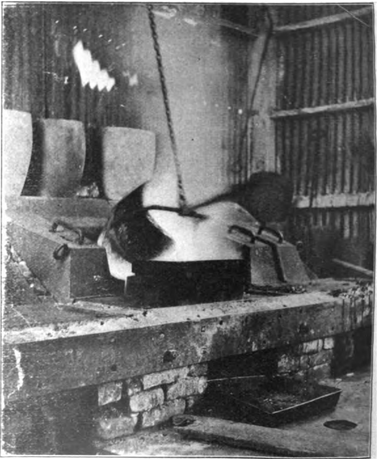
Pouring a 2300-ounce bar of gold-silver bullion at Standard Consolidated Mine, Bodie. Photo by Walter W. Bradley.
