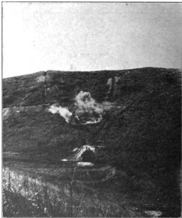
On the south of the Western Hill, of the Porterville Magnesite Company's property, showing main gash vein striking N. 45^{\circ} W., dip 70^{\circ} NE., width 2' to 8'.
