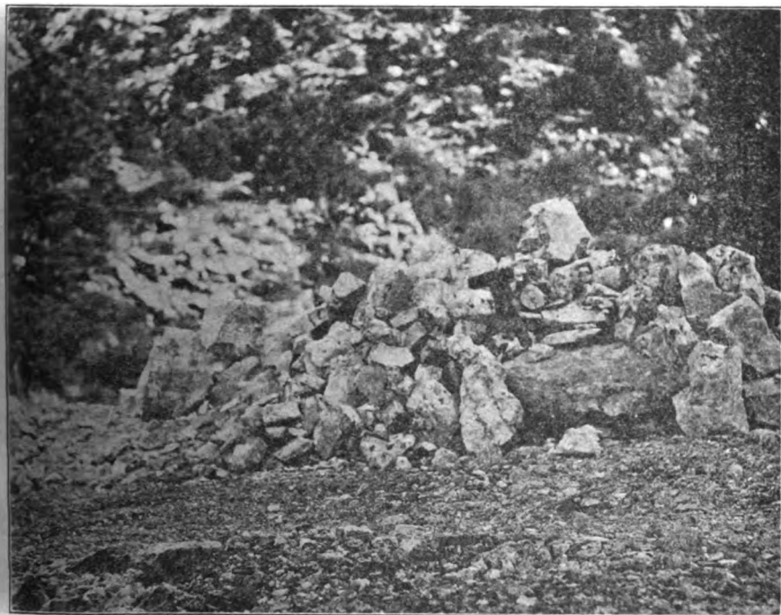
Photo No. 28. Tungsten ore at mouth of Carbonate tunnel. The wolframite shows as black spots in the rock.
