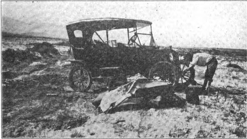
Photo No. 12. Using a "Pull-U-Out" attached to a "deadman," Amargosa Flat, near Saratoga Springs, Death Valley.
